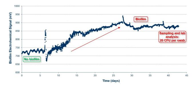
Thanks to the ALVIM technology, it was possible to see that the improved results provided by the new sanitation treatment could be considered only a first step towards the complete eradication of Legionella risk inside the Hospital's water system. Indeed, only keeping biofilm growth under control it is possible to maintain the risk of Legionella outbreaks as low as possible.
