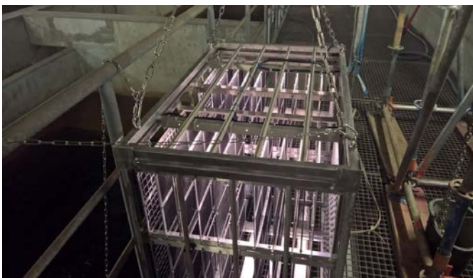
Fig. 1: Catalystmodule for once through applications with flow rates up to 2,500 m 3 /h
