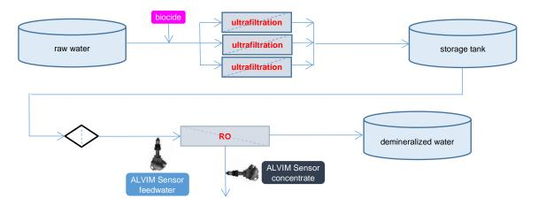
Figure 1: Scheme of the RO system
