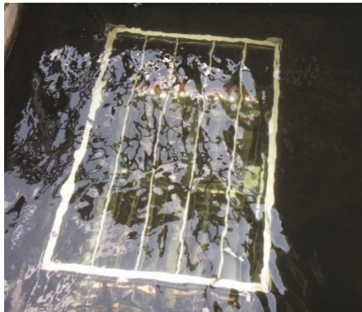
Fig. 5. MOLLIK-module installed at cooling basin
